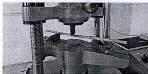
Figure 3: Load testing on full bamboo (O section)
